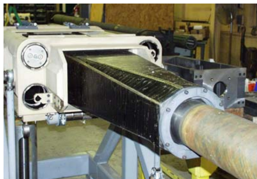
Figure 3: 105 MM MRAAS Tube with Composite Overwrap
